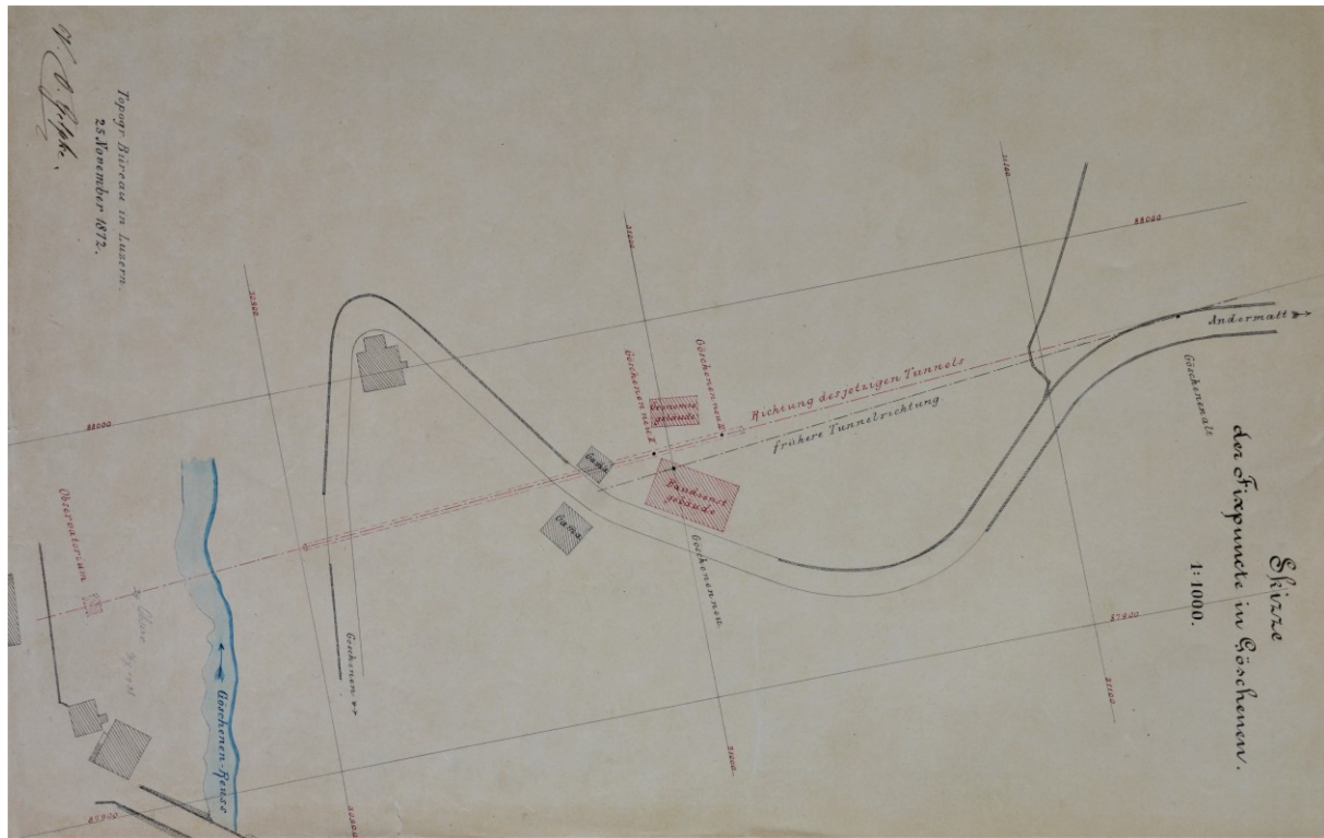
Abb. 20: Situationsplan Tunnelvisur, Göschenen, 1874 (SBB Historic, VGB_GB_SBBGB02_049_06)
